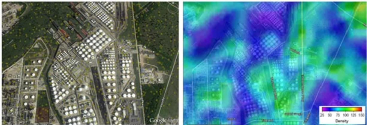
Figure 9. Individual lightning strikes plotted for an area in the Houston Ship Channel, Texas with filtered lightning density map covering the red area in Figure 4 in Houston, Texas.
