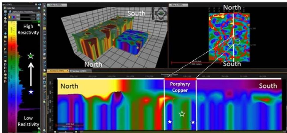
Figure 14. Probes, vertical, and horizontal resistivity slices from a resistivity volume at the Resolution Copper Mine porphyry deposit, Pinal County, Arizona. Innermost copper ore zone bounded by less resistive rock, possibly associated with hydrothermal alteration zones.
