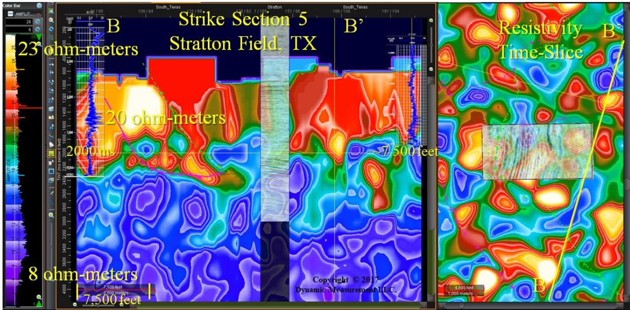
The seismic cross-sections below are overlaid with lightning derived apparent resistivity. Note how well the lightning high apparent resistivity fits within the seismic defined Vicksburg expansion fault.
