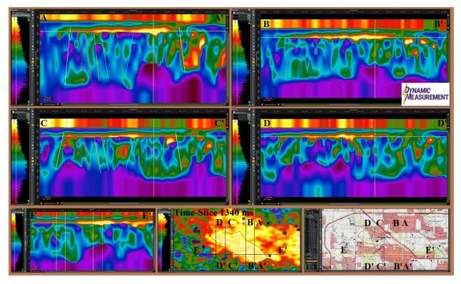
**#004 Lightning Houston Prospect.** Lightning analysis, unlike a 3-D seismic survey, is as easy to do in a big city as anyplace else. A typical project of 100 square miles has over 1 million lighting strikes. Above shows a shallow high apparent resistivity anomaly, probably natural gas, inside Beltway-8 in northwest Houston. This project data is from the 18 years of lightning strike data Dynamic Measurement has an exclusive license to for natural resource exploration.
